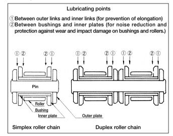
Lubricate on the sag side of the chain, i.e., at the position indicated in the following illustration. Since the lubricant is also useful for rust prevention, coating the entire surface of the chain with the oil is recommended.
