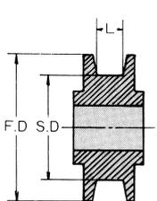
Minimum sheave diameter:  $S.D = \text{Chain pitch} \times 5$
